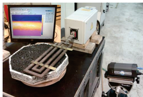
RSAT stone loss of Self Healing ZOAB sample plates with induction treatment after 12 hours
