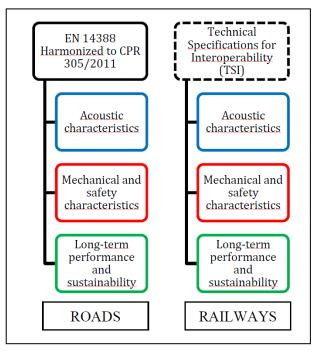
Figure 1. Main structure of the packages of standards for the road (on the left) and rail (on the right) sector.
