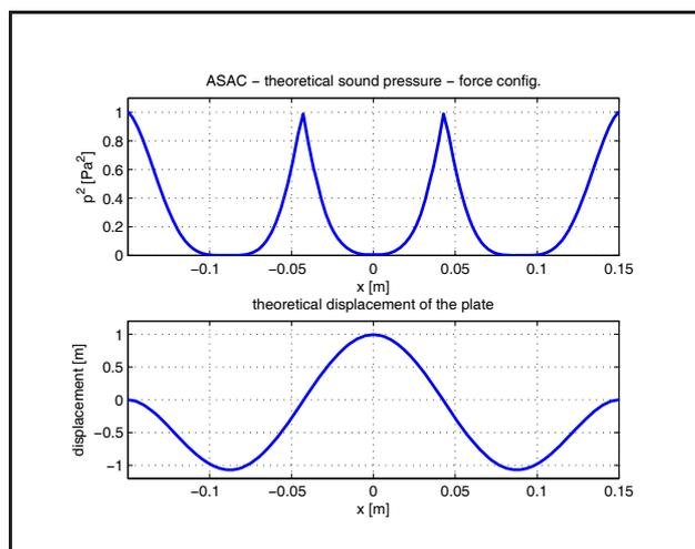
Figure 1. Normalized sound pressure at the microphone position for the force actuator.
