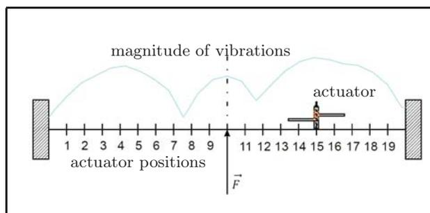
Figure 3. Measurement set-up with excitation force and positions of actuator.
