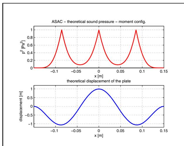
Figure 2. Normalized sound pressure at the microphone position for the moment actuator.
