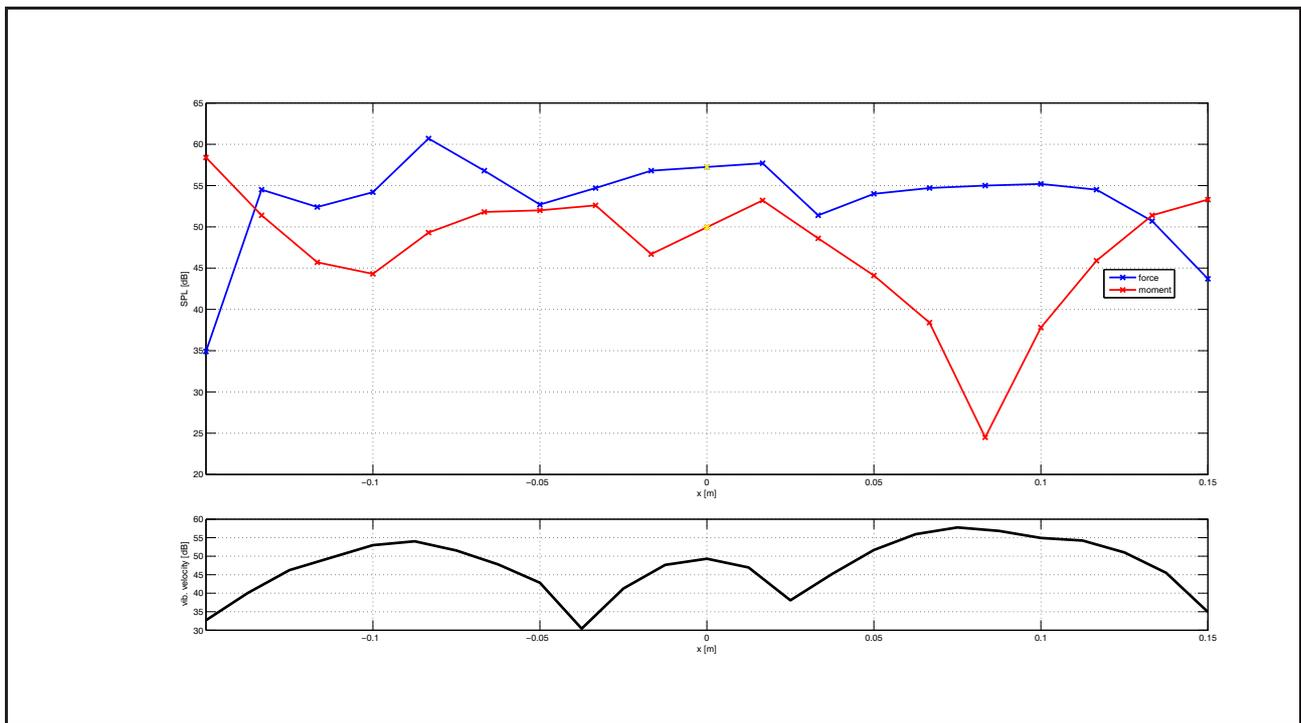
Figure 4. Sound pressure level generated by the actuator under the constant excitation.
