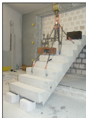
Figure 4. Stairs flight supported on the rigidly connected landing to the separating wall between the test rooms in Acoustics Laboratory of ITB
