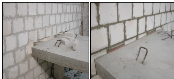
Figure 3. Model of landing connected to the separating wall between the test rooms in Laboratory of ITB (left: rigidly, right: by resilient elements)
