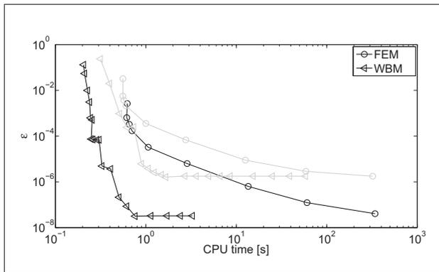
Figure 6. Convergence curves of the pore pressure at 250 (black) en 750 (grey) Hz. Finest adaptive FE model used as a reference.
