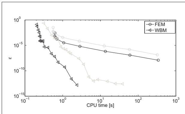
Figure 7. Convergence curves of the pore pressure at 250 (black) en 750 (grey) Hz. Finest WBM model used as a reference.
