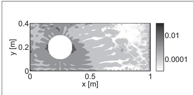
Figure 4. Logarithmic relative error  $\varepsilon(\hat{u}_x^s(\mathbf{r}))$  of the WBM model (555 DOFs) with respect to FEM (454,815 DOFs).
