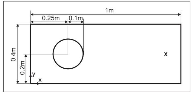
Figure 2. Rectangular poroelastic domain with a circular inclusion,  $x$  indicates the postprocessing point in which frequency response functions are calculated.
