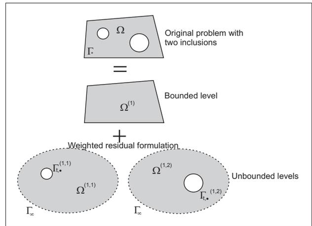
Figure 1. Illustration of the WBM Multi-Level concept.
