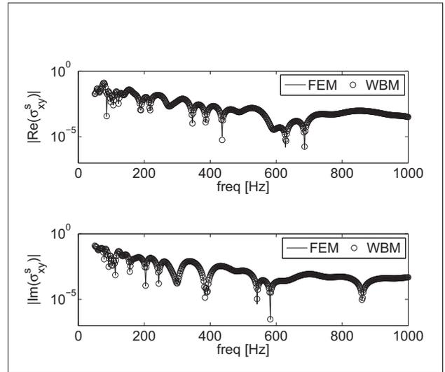
Figure 5. Frequency response function of the shear stress of the solid phase  $\sigma_{xy}^s$  evaluated in point (0.9,0.2) and calculated with the WBM and FEM.
