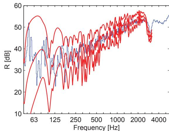
Figure 3. Sound transmission loss of a lightweight perforated brick wall. Predicted mean and 95% confidence interval, computed with the hybrid method (red), vs. laboratory measurements (blue).
