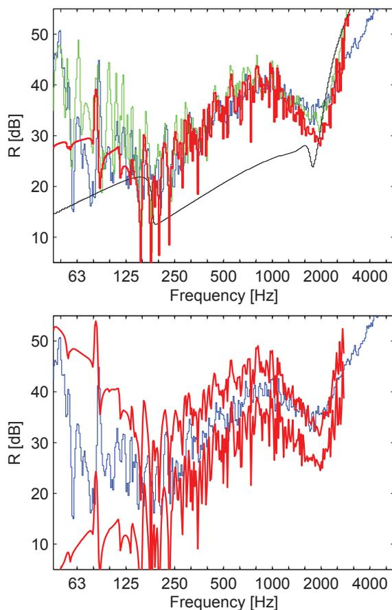
Figure 4. Sound transmission loss of double glazing 6–12–8 mm. (top) Predicted mean, computed with the hybrid method (red), vs. laboratory measurements (blue) and deterministic predictions with the TMM (black) and WBM (green) methods. (bottom)  $2\sigma$  confidence interval of the hybrid model predictions (red) vs. laboratory measurements (blue).
