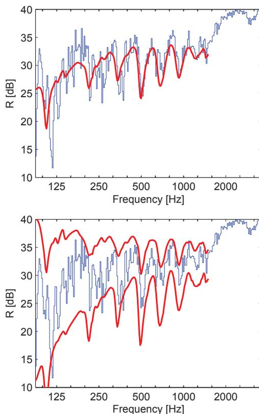
Figure 2. Measured sound reduction index of a rib-stiffened plate in 1/48-octave bands (blue) vs. the harmonic mean values (red, top) and 95% confidence intervals (red, bottom) as predicted with the hybrid method.
