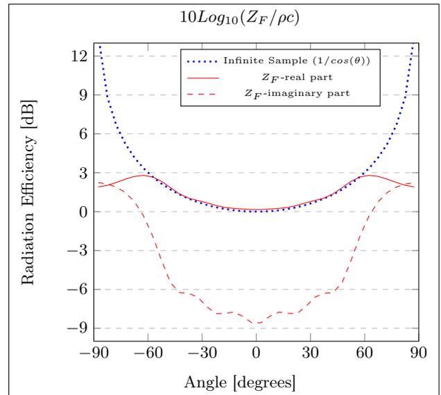
Figure 1. Logarithmic plot of the average normalized radiation impedance  $Z_F/\rho c$  at all angles of incidence for 1000 Hz. on a 1m x 1 m sample.
