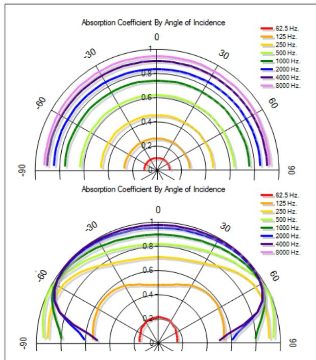
Figure 3. Polar plot of absorption from a 112 mm thick mineral wool, infinite sample (top), and 2.4 meter x 2.4 meter sample using equation (13). (bottom).
