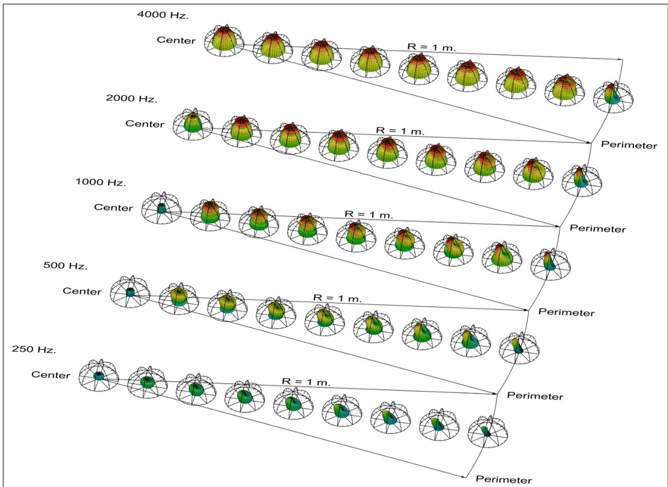
Figure 4. 3d Polar plot of absorption coefficient at various locations on a 2 m. diameter disc of 112 mm thick mineral wool, using equation (13), and averaged over each respective octave band shown.
