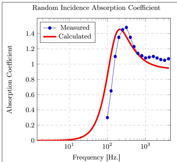
Figure 2. Plot of the random-incidence absorption coefficient, according to equation (9). Data is taken from section 12.3.3 in reference [3]. Calculated sample is a 2.4 m x 2.4 m sample of mineral wool calculated according to Miki's technique, with a flow resistivity of 15,000 mks-rays.
