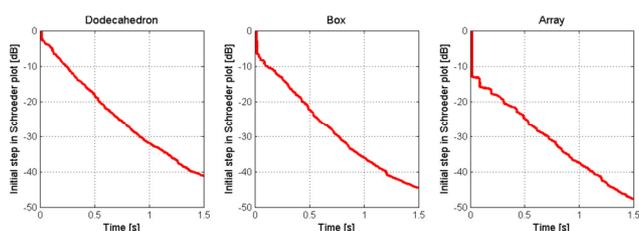
Figure 4. Example of three Schroeder plots measured in a sports hall at a distance of 5 meter from a dodecahedron (12 lsp's), a box (1 lsp) and a line array (7 lsp's).
