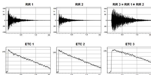
Figure 1. Example of the effect of 'room-in-room' acoustics on measured room impulse responses (RIR's) and energy time curves (ETC's) [2].
