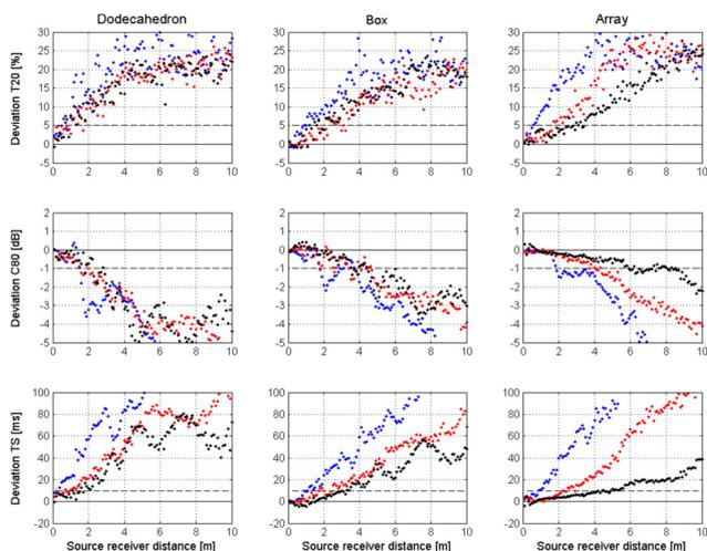
Figure 6. Difference between room acoustic parameter values of the recorded diffuse field room acoustics and the values for the same parameters when playing back the recorded acoustics in the
