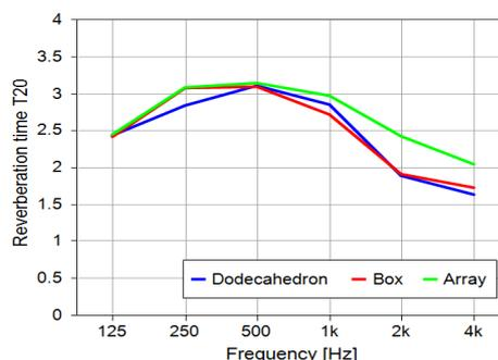
Figure 3. Reverberation time of the sports hall derived from all measurements, for each of the used sound sources.
