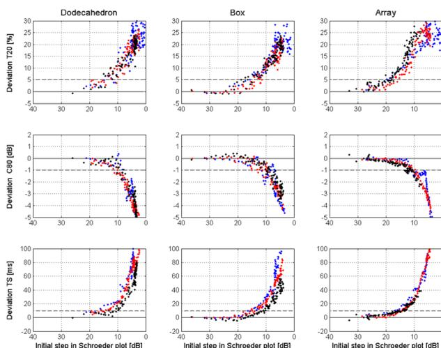
Figure 7. Difference between room acoustic parameter values of the recorded diffuse field room acoustics and the values for the same parameters when playing back the recorded acoustics in the same hall, presented as a function of the *initial drop value of the Schroeder plot*, sound source type and octave band: 500 Hz (blue), 1 kHz (red) and 2 kHz (black).
