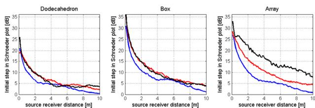
Figure 5. Initial drop value [dB] of the Schroeder plot as a function of the source-receiver distance and octave band: 500 Hz (blue), 1 kHz (red) and 2 kHz (black), for all three sound source types.
