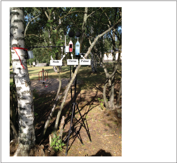
Figure 4. Node attachment and reference sound level meters
