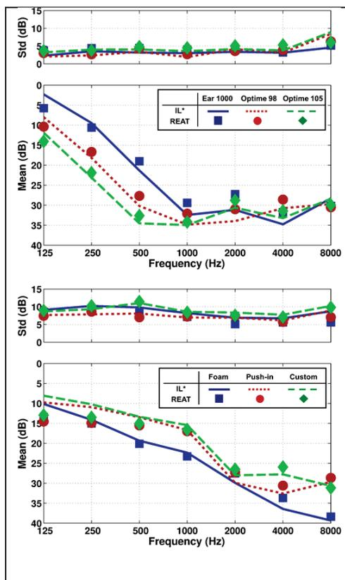
Figure 1: REAT and IL\* attenuation values (mean and standard deviation) for the earmuffs (upper) and the earplugs (lower) tested
