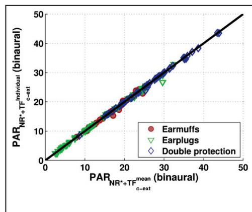
Figure 3: PAR results computed with NR\* corrected with individual  $TF_{c-ext}$  (ordinate) vs mean  $TF_{c-ext}$  values (abscissa).
