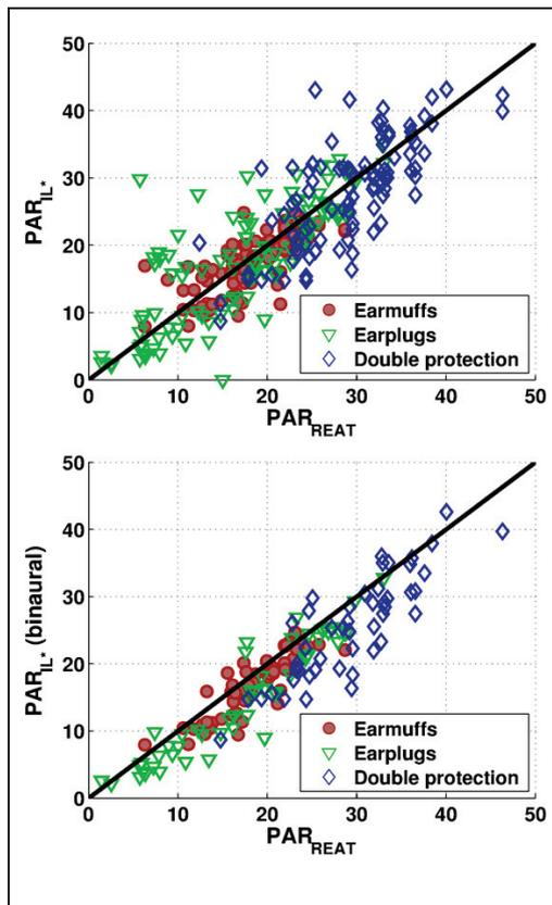
Figure 2: PAR values computed with IL\* compared to PAR computed with REAT for earmuffs, earplugs and double protection. PAR values calculated for left and right ear separately (upper) and PAR values calculated with equivalent binaural estimates (lower) are shown.
