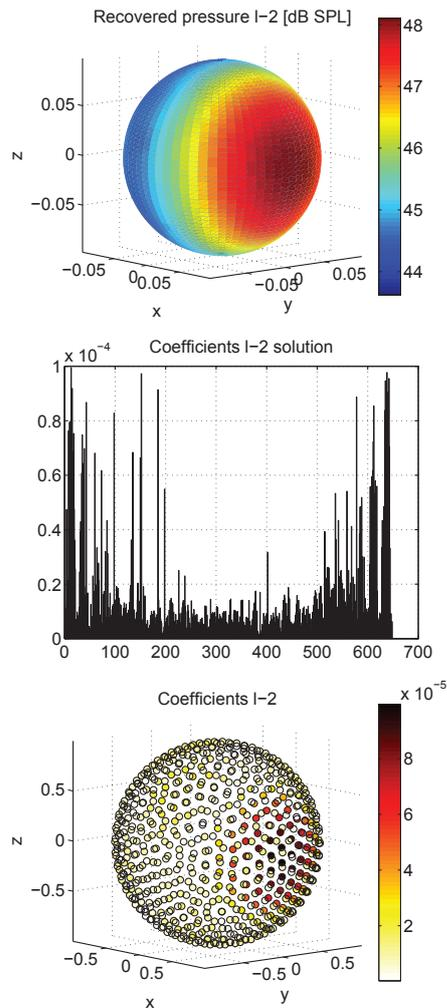
Figure 2. Spherical wave incident on a spherical array, expanded into plane waves (Eq. 2). Solution based on the  $l_2$ -norm - least squares (Eq. 8); Top: Recovered sound pressure; Mid: coefficients based on  $l_2$  minimization; Bottom: Coefficients ordered by their direction of arrival.
