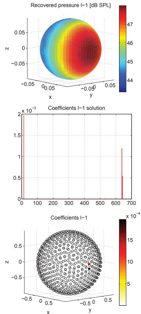
Figure 3. Spherical wave incident on a spherical array, expanded into plane waves (Eq. 2). Solution based on the  $l_1$ -norm - Compressive Sensing (Eq. 9); Top: Recovered sound pressure; Mid: coefficients based on  $l_1$  minimization; Bottom: Coefficients ordered by their direction of arrival.
