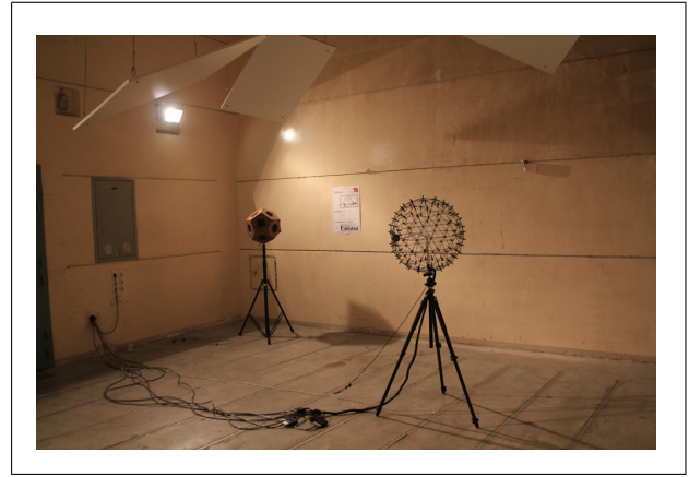
Figure 2. Measurement setup: microphone array and dodecahedron in the reverberation chamber.
