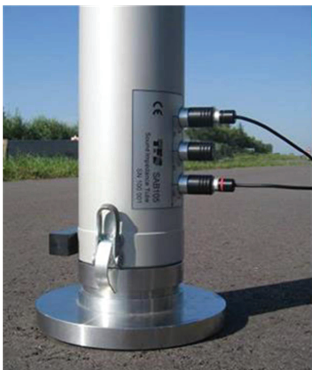
Figure 1. Impedance tube with fixture to measure the acoustic absorption of dense surfaces in situ. Top and bottom microphone position are used in this example
