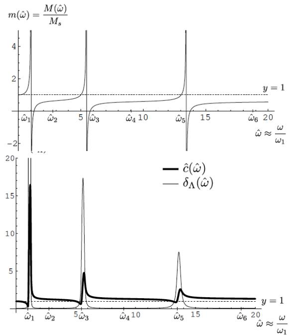
Figure 6. up: variation of the apparent mass induced by local resonance - down : variation of the velocity  $c$  and the associated attenuation  $\delta$  in case of low viscous damping.
