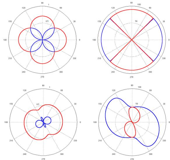
Figure 5. On top, case of the orthogonal inclined lattice ( $\varphi = \pi/2$ ) and below, lattice with an inclination of  $\varphi = \pi/4$ . On the left, the dimensionless velocities in function of the angle of propagation  $\phi$  (in degree) and on the right, the associated (blue or red) angle of polarization
