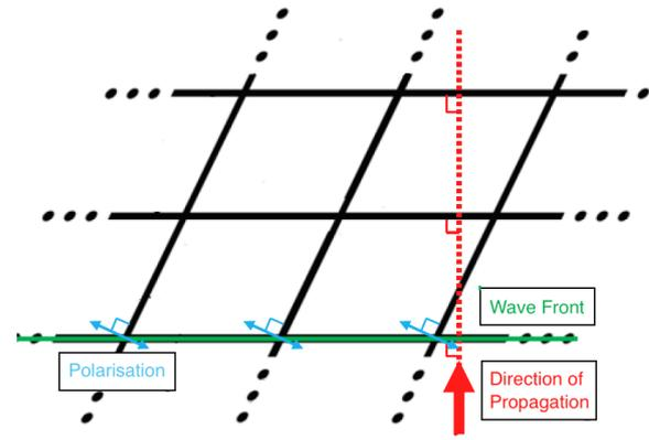
Figure 4. Shear wave traveling in the  $\pi/2$  direction ( $\alpha = \pi/2$ )
