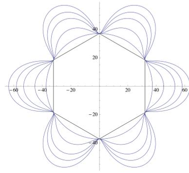
Figure 7. Profil of shear wave velocities in function of the direction of propagation and in function of the frequency. Results obtained on an aluminium honeycomb with the geometrical properties :  $\ell = 5.8$  mm,  $h = 23$  mm and  $a = 0.06$  mm. The bars represent the orientation of the honeycomb.
