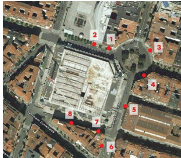
Figure 1. Receiver points used in the measurement campaign of noise levels caused by the global activity.
