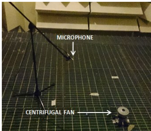
Figure 3: Centrifugal Fan Measured in semi anechoic chamber
