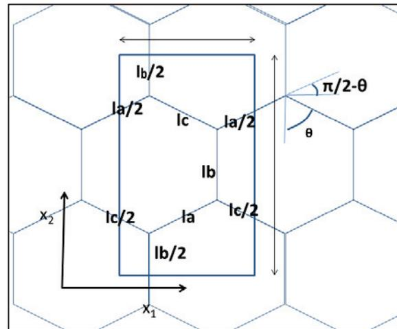
Figure 2. Struts in the unit cell used for calculating the flow resistivity, with notations and orientations. At the junctions a vertical strut is connected, which gives four vertical struts  $l_d$  aligned with the  $x_3$  axis in the unit cell.
