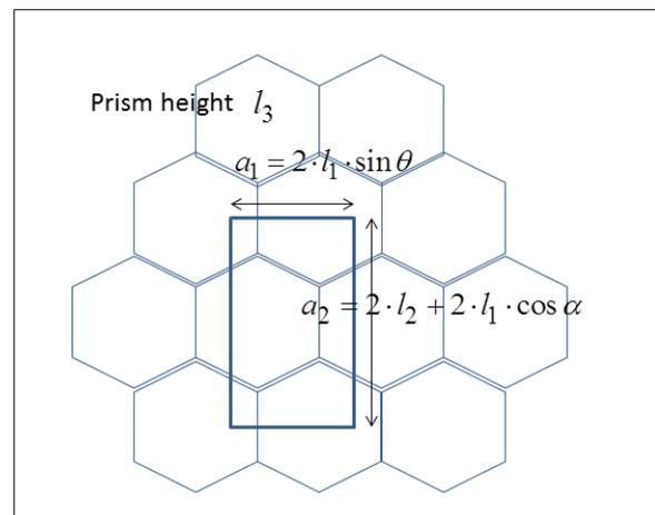
Figure 1. Micro model geometry in the plane  $x_1$ - $x_2$  for a periodic unit cell. The choice of unit cell is shown in the figure, together with the dimensions of the unit cell. The height of the unit cell is  $l_3$ .
