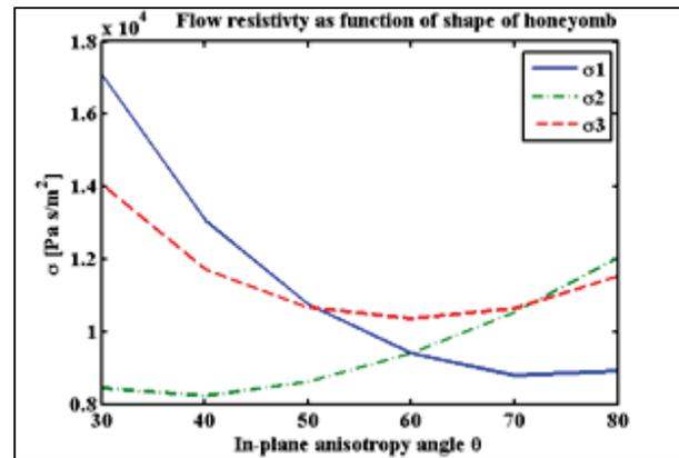
Figure 4. Calculated flow resistivity for a hexagonal micro-cell. The height of the PUC is approximately the same as the width. The average for a regular cell with  $\theta=60$  deg is  $9.7 \text{ kPa s/m}^2$ . The height is 80% of the in-plane strut length.
