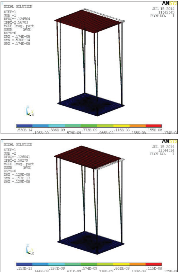
Figure 7. The two initial calculated modal shapes of the construction
