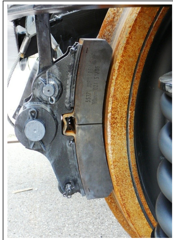
Figure 1. Freight wagon wheel with synthetic material brake Jurid 816M.
