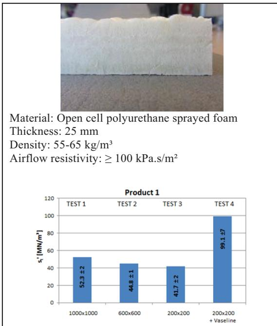
Figure 4. The average apparent dynamic stiffness for the open cell polyurethane sprayed foam for one sample and according to the four test procedures. The average and the standard variation are calculated on five measurements.
