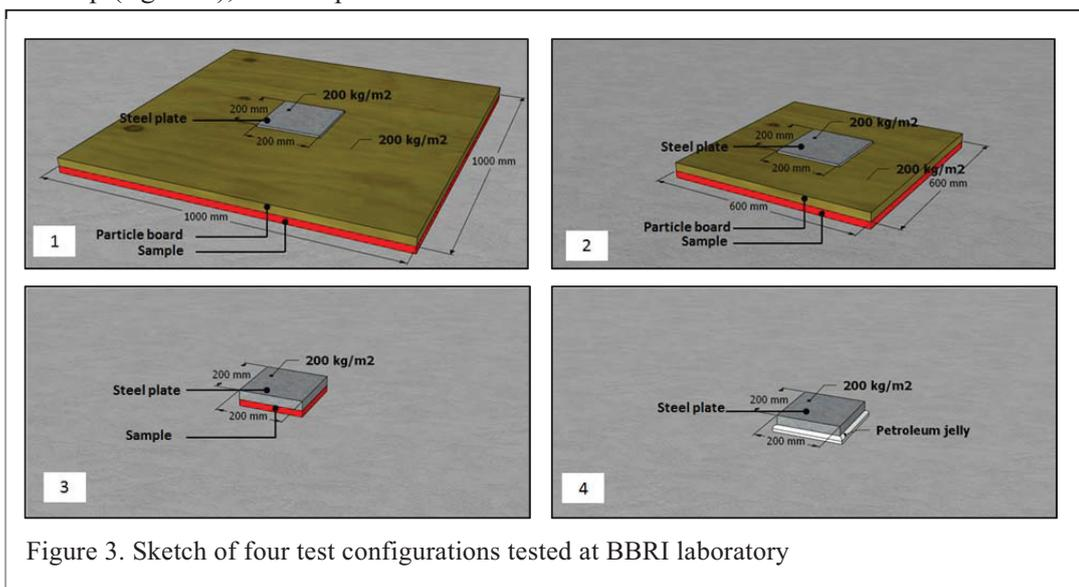
Figure 3. Sketch of four test configurations tested at BBRI laboratory
