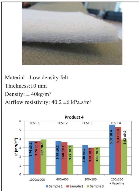
Figure 7. The average apparent dynamic stiffness for the low density felt for three samples (blue, red and green) and according to the four test procedures. The average and the standard variation are calculated on five measurements.
