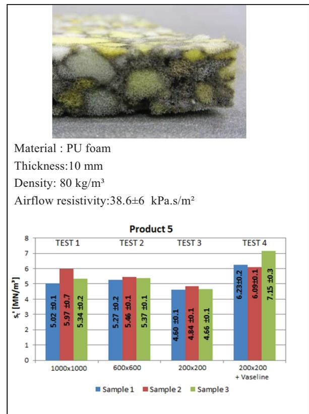
Figure 8. The average apparent dynamic stiffness for the PU foam for three samples (blue, red and green) and according to the four test procedures. The average and the standard variation are calculated on five measurements.
