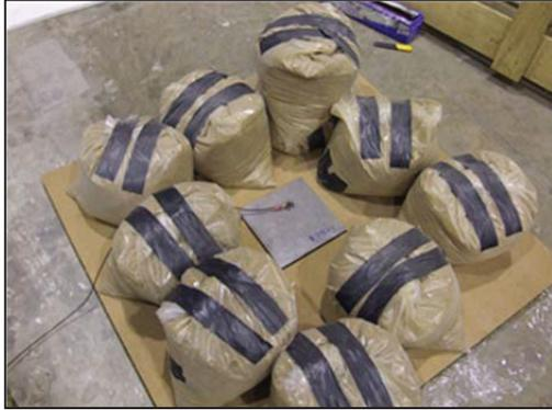
Figure 2. New test bench for the dynamic stiffness measurement
