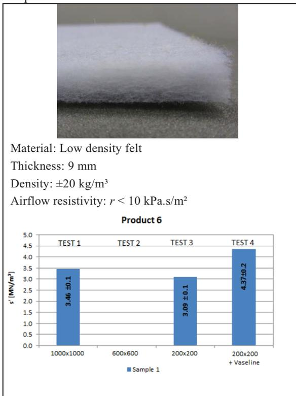
Figure 9. The average apparent dynamic stiffness for the Low density felt for one sample and according to three test procedures. The average and the standard variation are calculated on five measurements.
