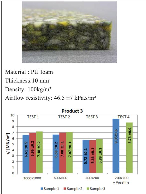
Figure 6. The average apparent dynamic stiffness for the PU foam for three samples (blue, red and green) and according to the four test procedures. The average and the standard variation are calculated on five measurements.
