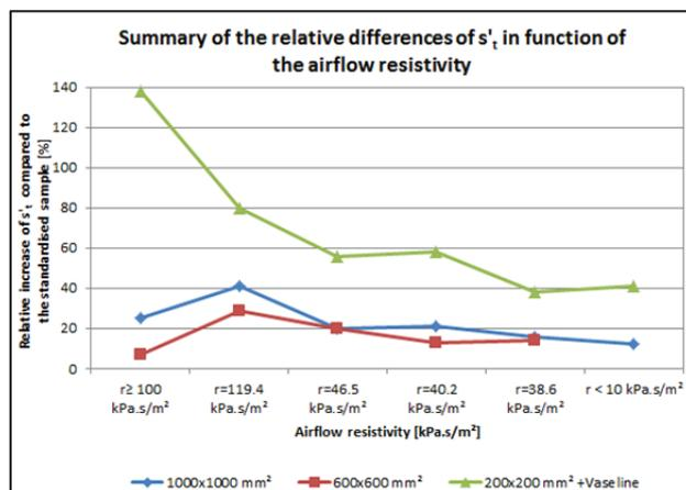
Figure 10. The average relative difference of  $s'_t$  in percentage compared to the standardised results of the standard ISO 9052-1 in function of the airflow resistivity. (In blue, the results for the 1000x1000 mm<sup>2</sup> samples, in red, the results for the 600x600 mm<sup>2</sup> samples and in green the results for the 200x200 mm<sup>2</sup> samples with Petroleum jelly).
