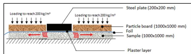
Figure 1. Diagram of the general principle
