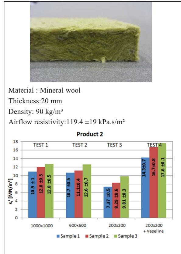
Figure 5 – The average apparent dynamic stiffness for the mineral wool for three samples (blue, red and green) and according to the four test procedures. The average and the standard variation are calculated on five measurements.
