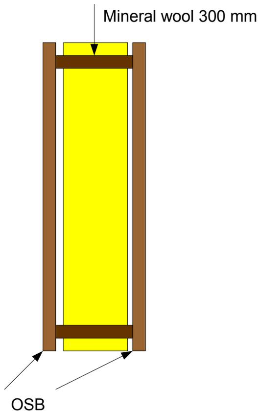
Figure 8. Basic facade element
