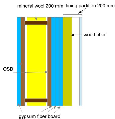
Figure 11. Thinner facade element and lining partition
