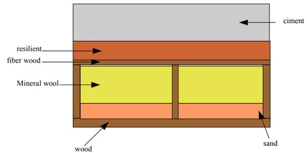
Figure 4. Floor structure with a wet floating floor
