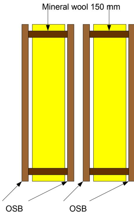
Figure 6. Double partition using two basic elements
