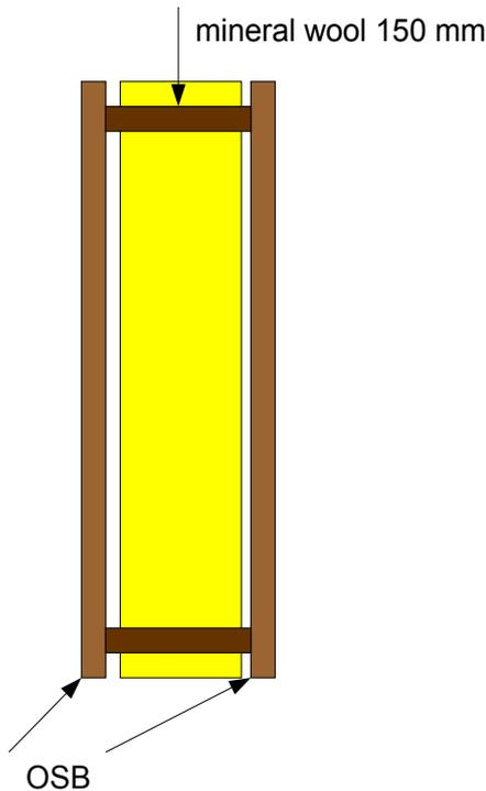
Figure 5. Basic wall element
