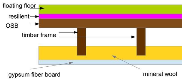
Figure 1. Usual floor construction to meet the NBN S01-400-1 requirements
