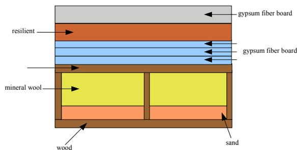
Figure 3. Floor structure with a dry floating floor
