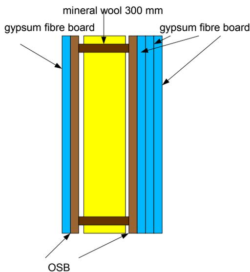
Figure 9 . Complete facade element
