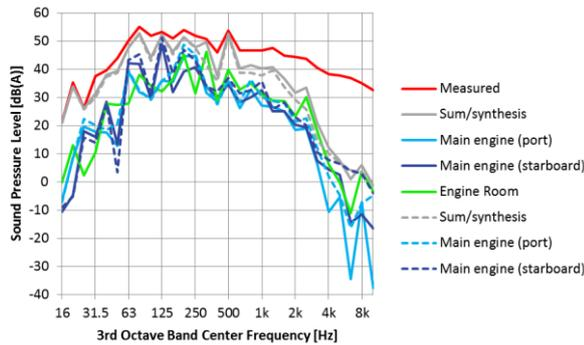
Figure 5. Contributions of the main engines to the sound pressure spectrum in the mess room for free sailing condition for OTPA analysis I (dashed) and analysis II (solid).
