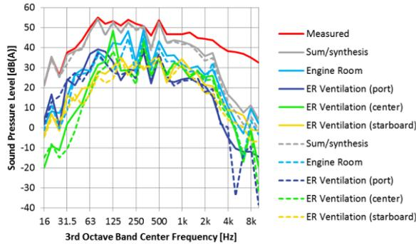
Figure 9. Contributions of the air borne sources to the sound pressure level in the mess room for free sailing condition for analysis III using high resolution transfer functions.
