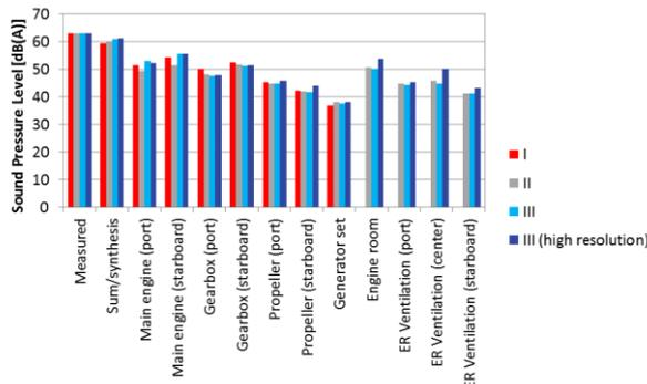
Figure 10. Comparison of the calculated contributions to the sound pressure level in the mess room for free sailing condition for all four OTPA analyses.
