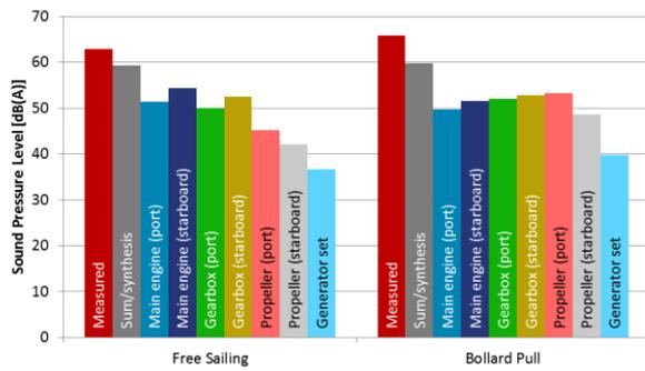
Figure 2. Contributions of the selected sources to the sound pressure level in the mess room for free sailing and bollard pull condition for OTPA analysis I.
