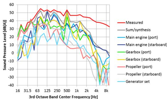
Figure 3. Contributions of the selected sources to the sound pressure spectrum in the mess room for free sailing condition for OTPA analysis I.
