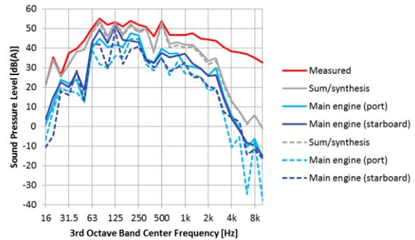
Figure 7. Contributions of the main engines to the sound pressure spectrum in the mess room for free sailing condition for OTPA analysis II (dashed) and analysis III (solid).
