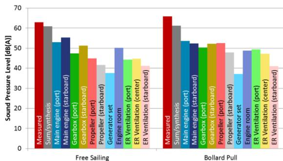
Figure 6. Contributions of the selected sources to the sound pressure level in the mess room for free sailing and bollard pull condition for OTPA III.
