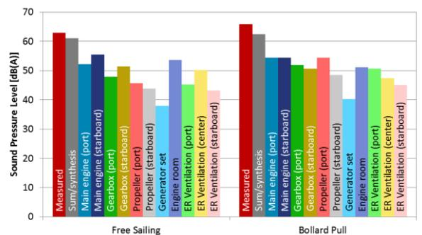
Figure 8. Contributions of the selected sources to the sound pressure level in the mess room for free sailing and bollard pull condition for analysis III using high resolution transfer functions.
