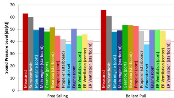
Figure 4. Contributions of the selected sources to the sound pressure level in the mess room for free sailing and bollard pull condition for OTPA analysis II.
