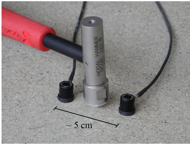
Figure 1. Experimental setup at each excitation point. The force was applied with an impulse hammer between a pair of accelerometers.
