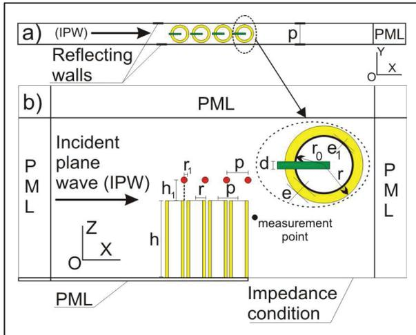
Figure 2. Comprehensive model where the real 3D problem is replaced by two 2D cases; (a) MP-model (OXY), which includes BG, resonances and absorption phenomena; (b) DIF-model (OXZ) with the main geometrical parameters of the problem considered. The PMLs and the impedance condition defined at the boundaries are also indicated in the figure. In the inset, one can see the main geometrical parameters of the multi-phenomena cylindrical scatterers.
