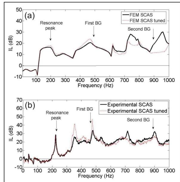
Figure 3. Attenuation results calculated behind the considered SCAS. (a) Numerical and (b) Experimental IL spectra respectively at the tested point with (red dotted line) and without (black continuous line) the tuned solution proposed to reduce diffraction at the upper edge of the device. The real value of the total pressure,  $\text{Re}(P)$ , is plotted in both cases.
