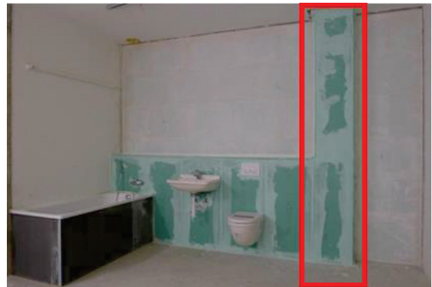
Figure 8. Sanitary installation system in a building-like test rig with additional installation shaft enclosing the waste water pipe.
