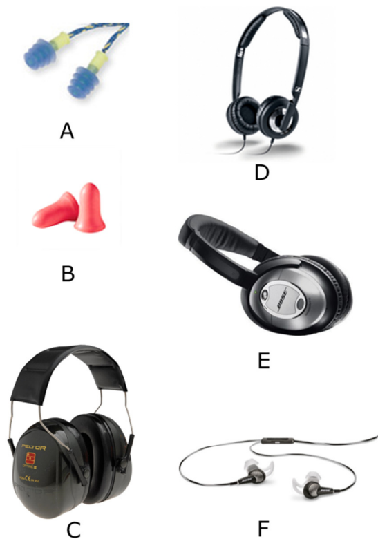
Fig.5 DUT's: Hearing protection devices: In ear Soft flange (A), In ear Foam (B), Circum-aural (C). Headphones: Supra-aural (D), Circum-aural (E) and In-ear (F).
