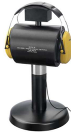
Fig.3 ATF (45CA) According to ISO 4869-3
