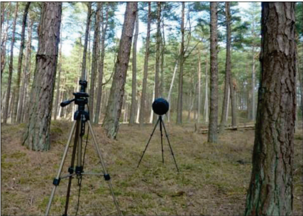
Picture 3. Measuring impulse response in pine forest.
