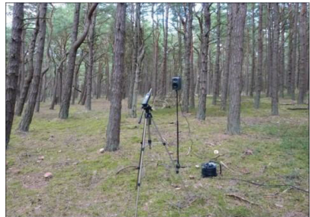
Picture 1. Measuring sound level at 1 meter.
