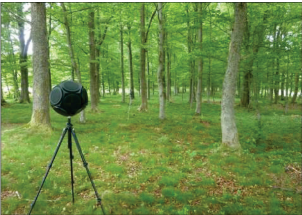
Picture 5. Measuring impulse response in beech forest.
