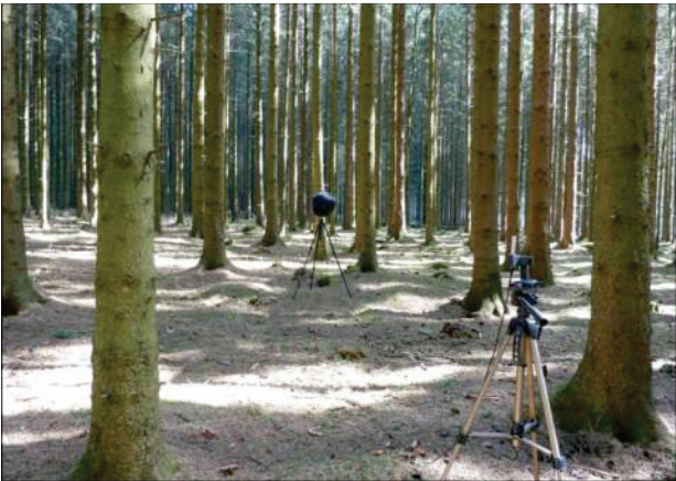
Picture 4. Measuring impulse response in fir forest.
