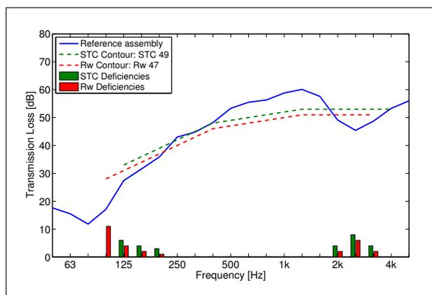
Figure 2. Sound Transmission Loss of reference assembly: G16\_SS152(406)\_GFB152\_RC13(406)\_G16
