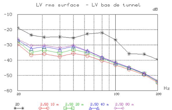
Figure 4. Case 1: soil attenuation for 2D and 2.5D models (1/3 octave bands).
