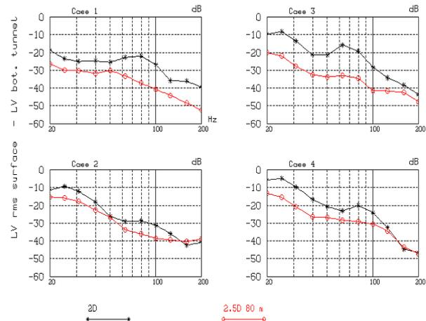
Figure 5 . 4 cases: soil attenuation for 2D and 2.5D models.
