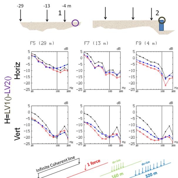
Figure 2. Surface insertion loss. 2D versus 2.5D
