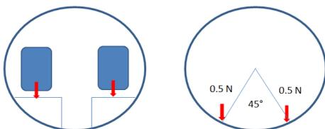
Figure 3. A tunnel with two trains and the corresponding excitations.
