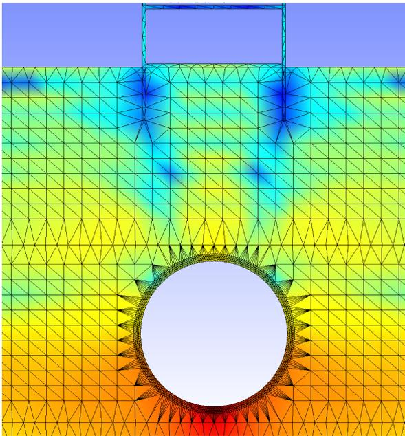
Figure 10. zoom with calculation and post-treatment meshing (2D)
