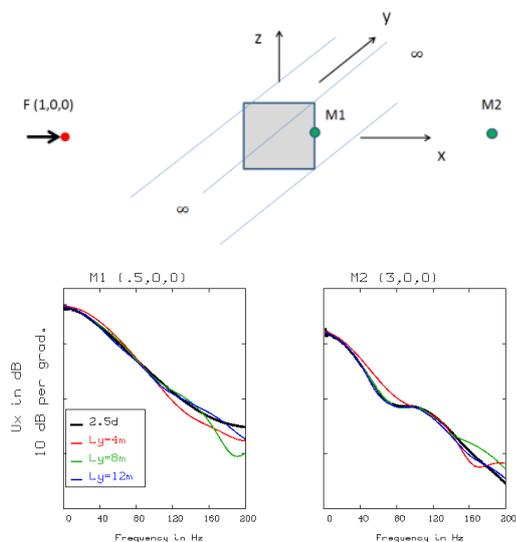
Figure 1. Comparison of 2.5D and 3D computations
