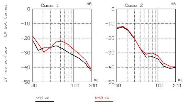
Figure 8. Effect of the tunnel's walls' thickness (2.5D).
