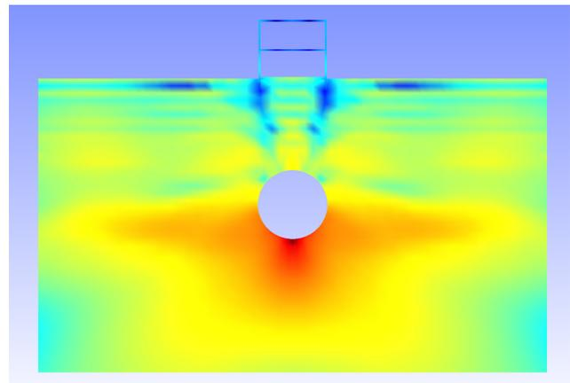
Figure 9. Total displacement at 100 Hz. Color span of 38 dB (2D)
