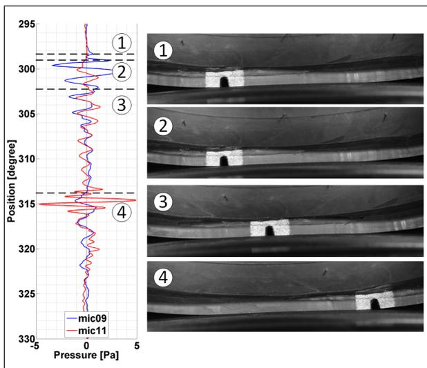
Figure 7. Synchronous image and microphone data
