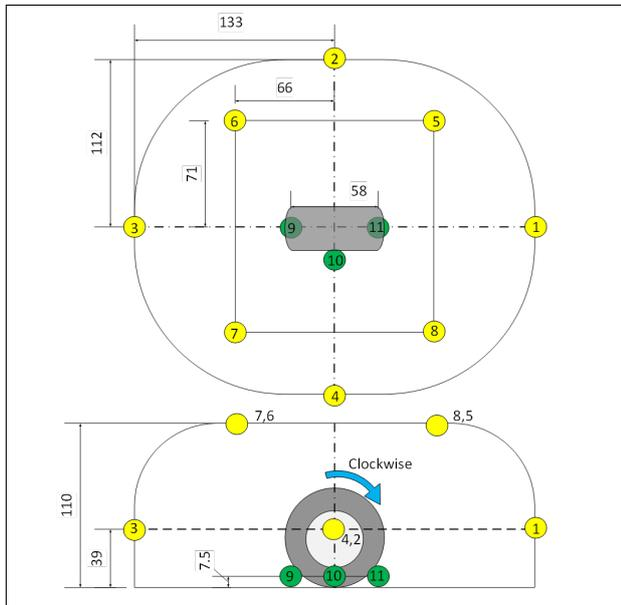
Figure 4. Microphone placement in centimeter
