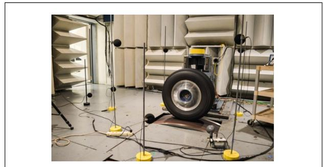
Figure 5. Semi-anechoic chamber testing facility
