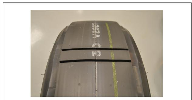
Figure 6. Hand cut tire with two slots
