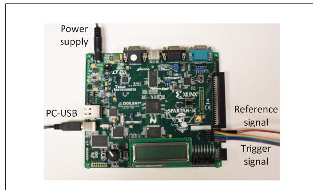
Figure 2. Visualization system implemented in a FPGA development board
