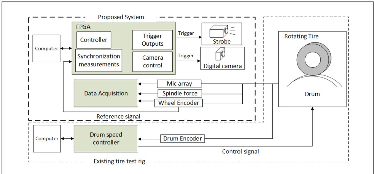
Figure 1. Overall system schematic
