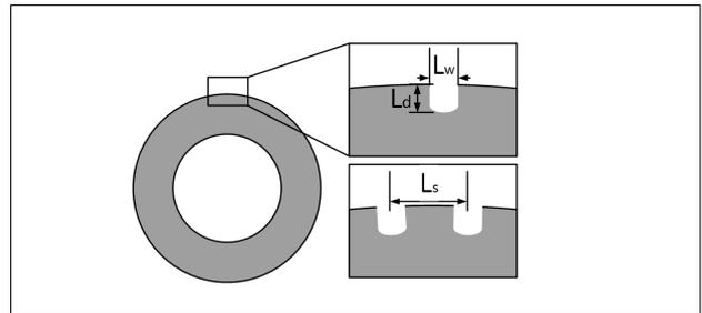
Figure 3. Tire slot dimensions
