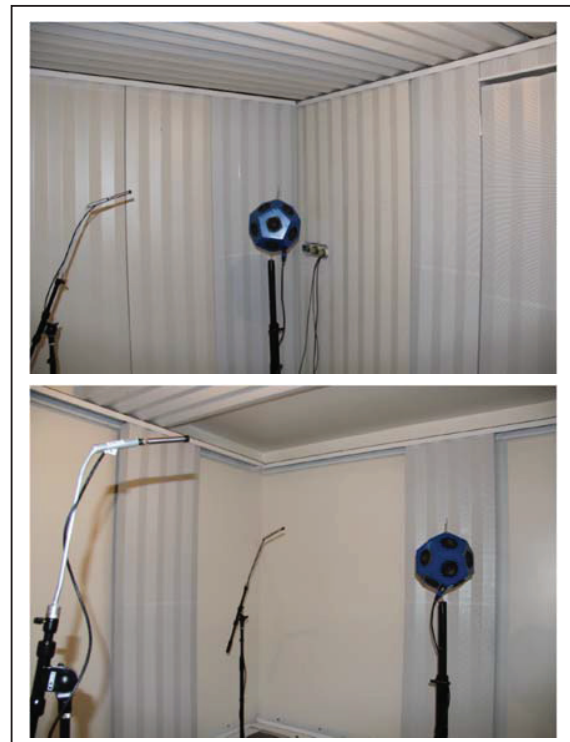
Figure 2. Variable Acoustics Chamber without visually opaque grill cloth showing two reverberation conditions. Upper, low reverberation condition at 0.2 sec; Lower, medium reverberation at 0.5 sec.
