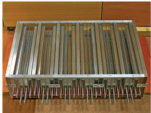
Figure 2 Tested sound diffuser with regulated wells' depths
