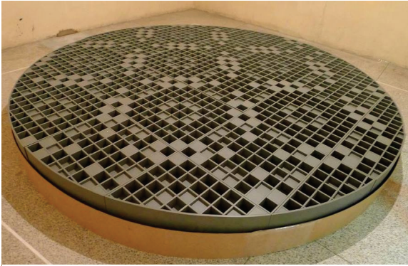
Figure 1 Tested sound diffuser in reverberation chamber
