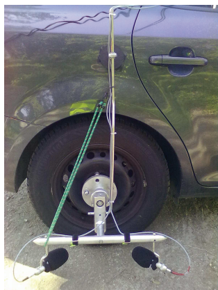
Figure 2. Tyre-road noise measurement set up.
