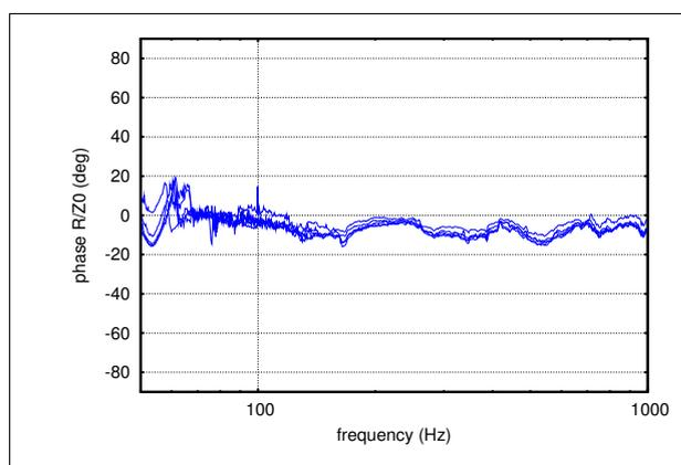
Figure 6. Phase of the slit resistance in terms of frequency for different loudspeaker excitation levels.
