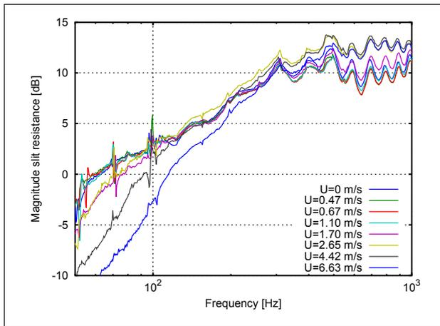
Figure 12. Slit resistance in terms of particle velocity through the slit for different frequencies (thick red lines: measured, thin blue lines: simulated using expression (18))
