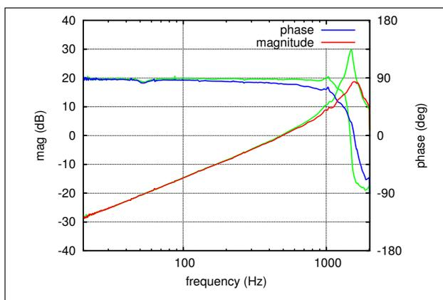
Figure 4. Comparison of the impedance of the device with open slit in magnitude (red line), (reference 0dB=  $Z_0$ ) and phase (blue line) and the impedance with closed slit (green line).
