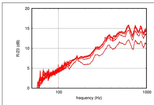
Figure 5. Magnitude of the slit resistance in terms of frequency for different loudspeaker excitation levels. Lowest curve: 10V, curve above 20V and so on for 30V, 60V to the upper curve 100V.
