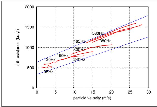
Figure 7. Slit resistance in terms of particle velocity through the slit for different frequencies (thick red lines: measured, thin blue lines: simulated using expression (18))
