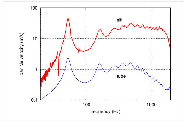
Figure 10. Particle velocity  $u_0$  before the slit (thin blue line) and  $u_s$  through the slit (thick red line) while contracting from the surface  $S_0$  to  $S$  with a loudspeaker excitation level of 100V.
