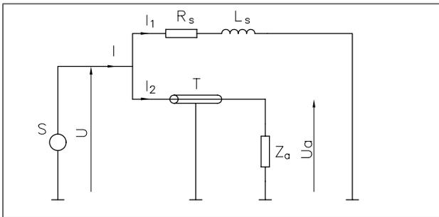
Figure 3. Electrical equivalent circuit of the damping device.
