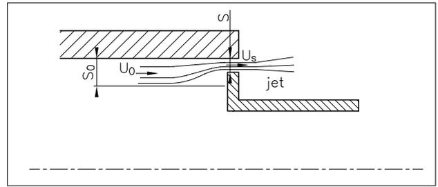
Figure 9. Contraction of the flow through the slit.
