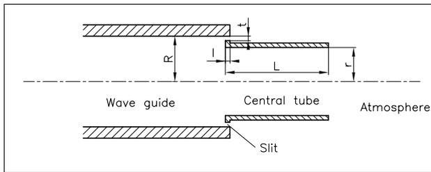
Figure 1. Scheme of the damping device.
