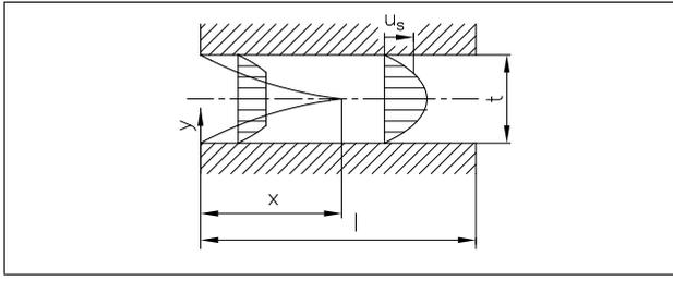
Figure 11. Velocity distribution in the slit during formation of hydrodynamic developed flow.
