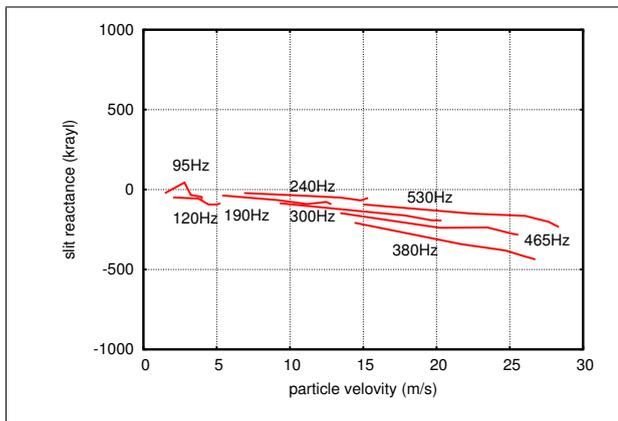
Figure 8. Measured slit reactance in terms of particle velocity through the slit for different frequencies.
