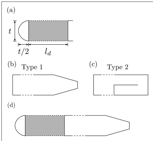
Figure 2. Diagram showing the shape along the axis of (a) a dissipative element, (b) a type 1 reactive element, (c) a type 2 reactive element and (d) a hybrid silencer baffle formed by combining a reactive and dissipative element.
