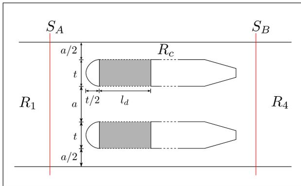
Figure 1. Diagram showing a plane along the duct system. Dashed lines represent perforated plates while shaded areas represent porous material.
