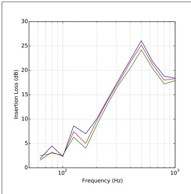
Figure 8. Measured insertion loss of S3 in flow with speeds of  $0\text{ms}^{-1}$  (—),  $13\text{ms}^{-1}$  (—) and  $26\text{ms}^{-1}$  (—).
