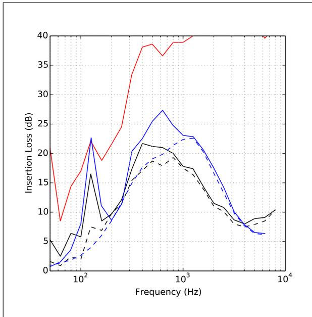
Figure 4. Insertion loss of S1 (Measured, - - -; Predicted, - - -) and S2 (Measured, —; Predicted, —). Limiting insertion loss, —.
