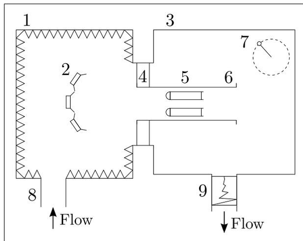
Figure 3. Diagram of equipment showing the anechoic chamber (1), the loudspeaker array (2), reverberation room(3), separating wall (4), silencer (5), test duct (6), microphone on rotating arm (7), flow inlet duct (8) and flow exit duct with silencer (9).
