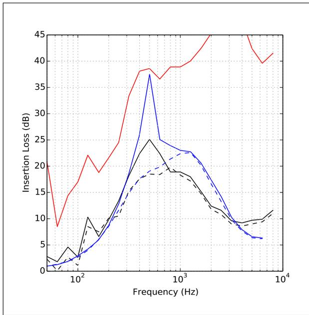
Figure 5. Insertion loss of S1 (Measured, - - -; Predicted, - - -) and S3 (Measured, —; Predicted, —). Limiting insertion loss, —.
