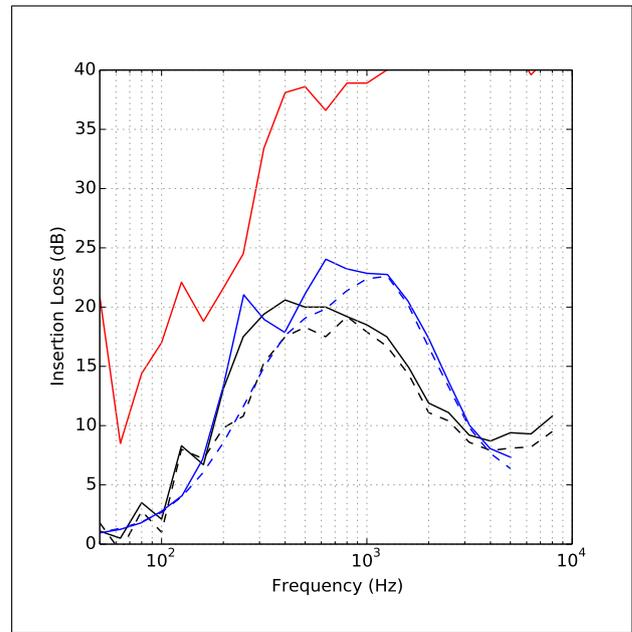
Figure 7. Insertion loss of S1 (Measured, - - -; Predicted, - - -) and a silencer using 1 baffle of S4 and S5 (Measured, —; Predicted, —). Limiting insertion loss, —.
