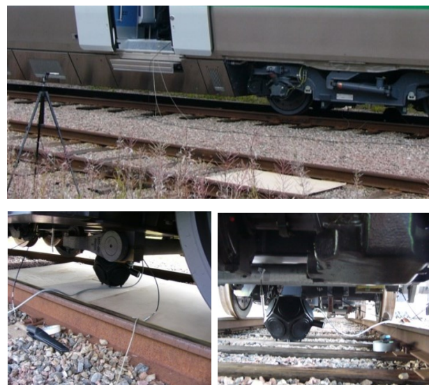
Figure 2. Measurement set-up with omnidirectional loud speaker in a bogie centre, top: receiver position at 7.5 m, left: plywood cover as concrete slab imitation, right: ballast track configuration
