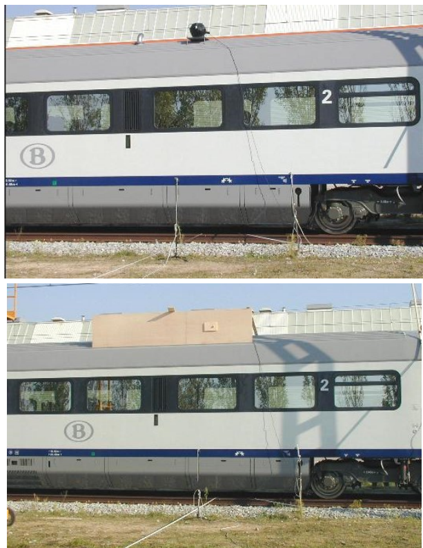
Figure 7. Measurement setup for transfer function measurements on a real train, above: w/o screen, below: with screen
