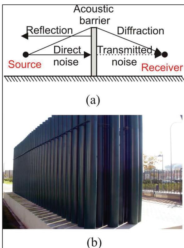
Figure 1. (a) Performance of an Acoustic Barrier; (b) An example of Sonic Crystal Acoustic Screen (SCAS).
