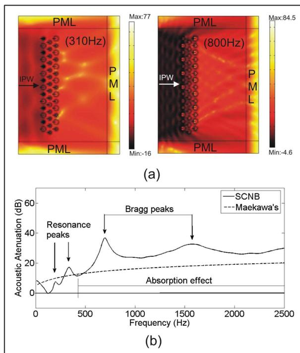
Figure 3. Theoretical simulations: a) Attenuation maps for 310Hz and 800Hz; b) Attenuation spectrum ( $0^\circ$  incidence) measured 1m behind the end of the SCAS.
