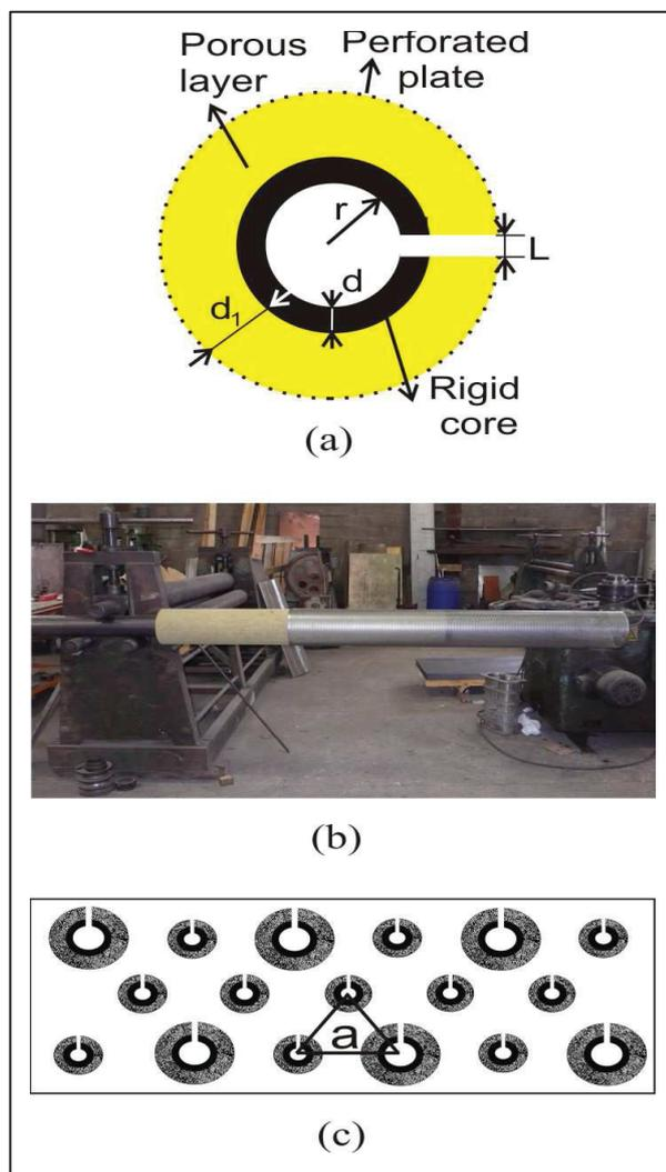
Figure 2. SCAS design and construction: (a) Cross section of the multiphysical scatterer designed; (b) Assembly of the three elements of the scatterers (rigid core, porous layer and perforated plate); (c) Triangular arrangement of the Multiphysical scatterers.
