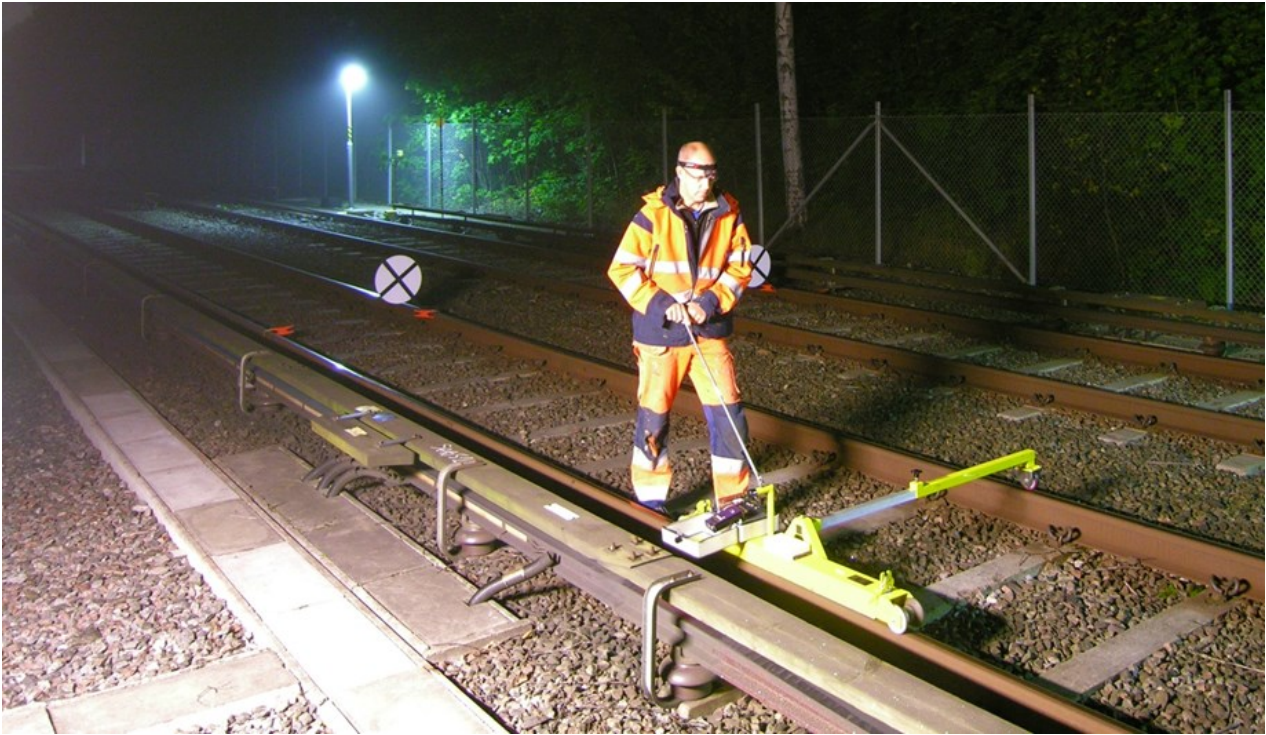
Figure 7. Measurement of track roughness using a rail surface analyser (RSA) from APT.
