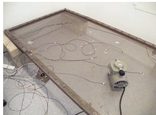
Figure 2: Air pump attached to the perforated plate
