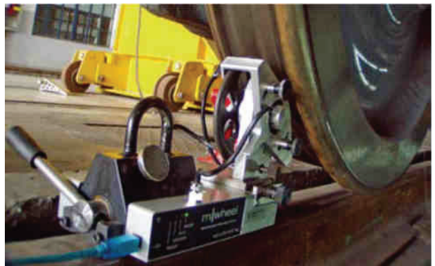
Figure 2. example of wheel roughness measurement device
