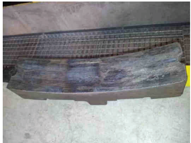
Figure 1. photo of a conditioned brake-block
