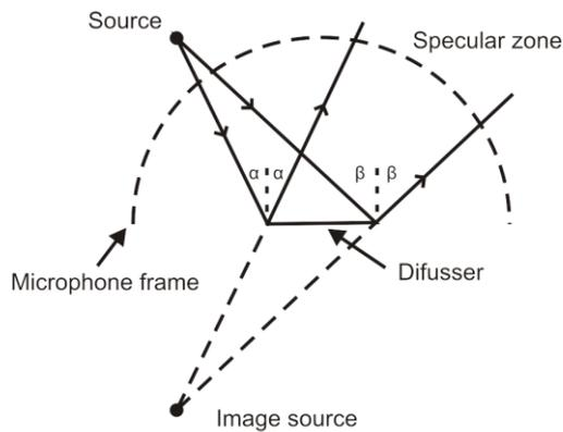
Figure 1. The schematic representation of the specular zone.
