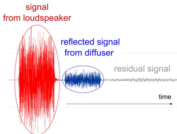
Figure 5. The time record of the measured signal recorded during real measurement in the hall.
