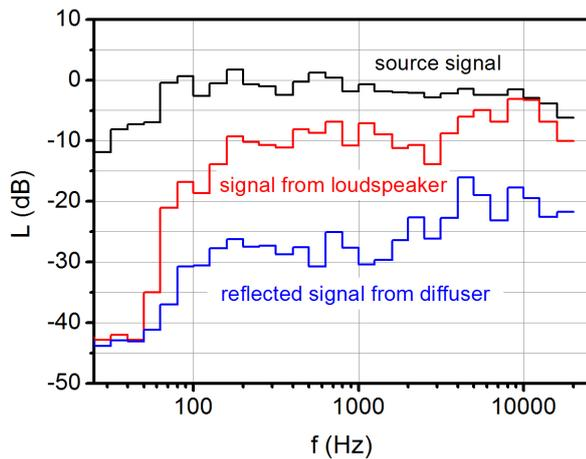
Figure 4. Measured frequency distribution of the power spectral density during real measurement in the hall.
