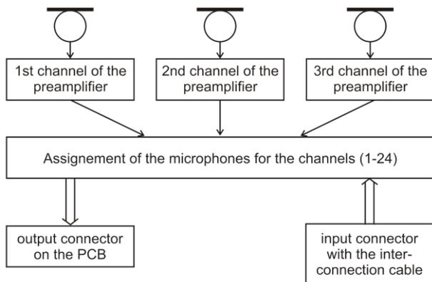
Figure 3. The block diagram of the electronics in one part of the microphone frame.
