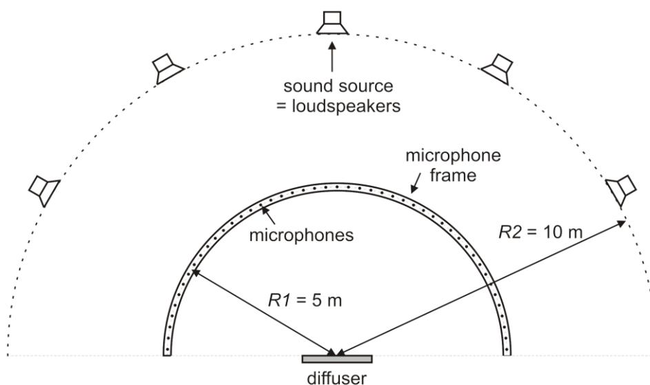
Figure 2. The scheme of the measurement system for the characterization of the diffuser with the size  $600 \times 600$  mm.
