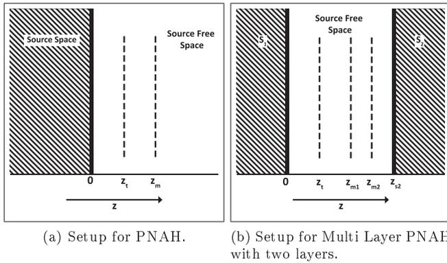
Figure 1: Side views of measurement setups for both PNAH and MLPNAH
