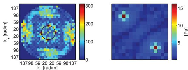
(b) Averaging of  $k_z$  reduces singularities in k-space (left) resulting in a more accurate reconstruction (right).
