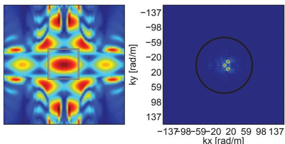
(c) Aperture (rectangle) expanded four times with LPBP (left) and corresponding k-space (right). All three peaks are visible in k-space.
