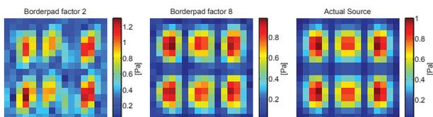
Figure 3: Reconstruction of vibrating plate with plane wave disturbance. Border padding factor of 2 (left) and 8 (middle) compared with actual source (right). Each point in these images represents the corresponding sensor.
