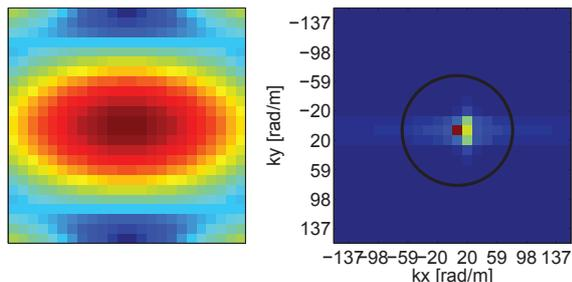
(b) Measured aperture (left) and corresponding k-space (right). Only a single peak is visible in k-space.
