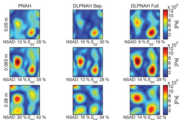
Figure 5: Measurement 1 results for front plane position 0.05, 0.065 and 0.08 m. Two point sources are located in front of the measurement planes.
