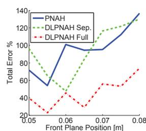
Figure 13: Total reconstruction error vs front plane position for measurement 3.
