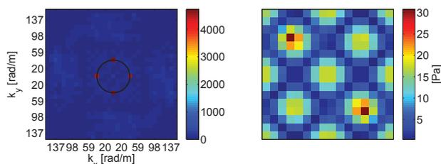
(a) Singularity in k-space pressure bins (left) on the radiation circle cause the reconstruction (right) to fail.
