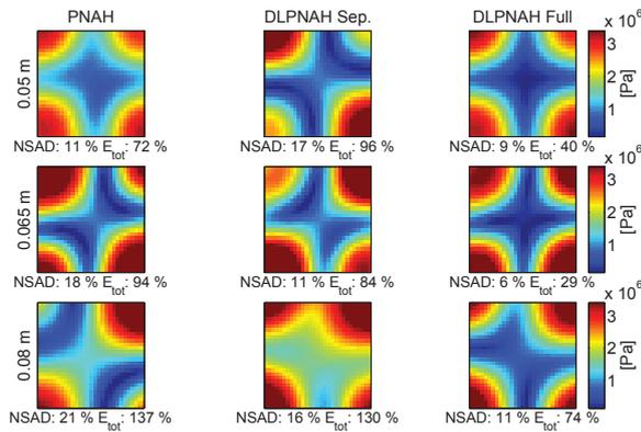
Figure 11: Measurement 3 results for front plane position 0.05, 0.065 and 0.08 m. A vibrating plate is located in front of the measurement planes and a point source is located behind the measurement planes.
