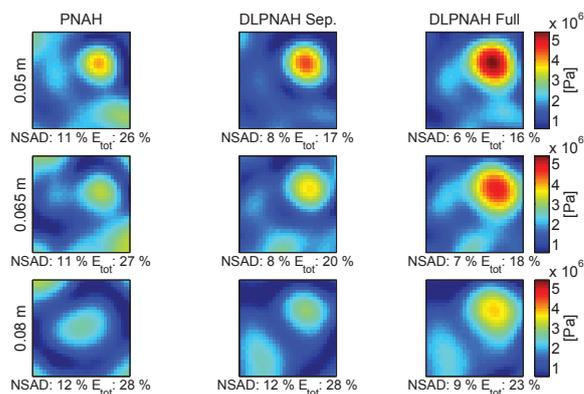
Figure 8: Measurement 2 results for front plane position 0.05, 0.065 and 0.08 m. One point source is located at the top right in front of the measurement planes and one at the bottom left behind the measurement planes.
