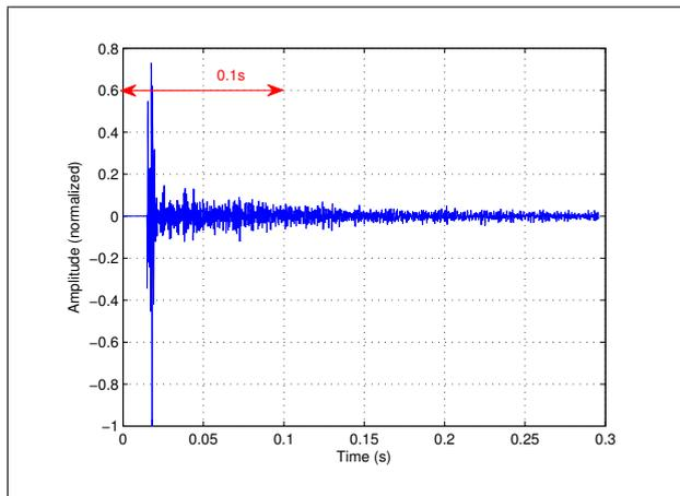
Figure 1. Typical detonation signal recorded at +/- 100 m from the source
