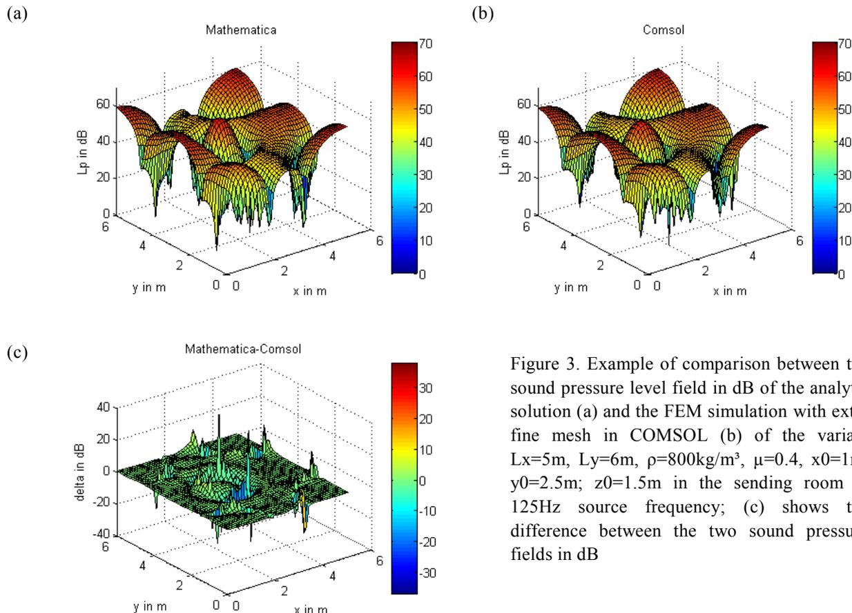
Figure 3. Example of comparison between the sound pressure level field in dB of the analytic solution (a) and the FEM simulation with extra fine mesh in COMSOL (b) of the variant  $L_x=5\text{m}$ ,  $L_y=6\text{m}$ ,  $\rho=800\text{kg/m}^3$ ,  $\mu=0.4$ ,  $x_0=1\text{m}$ ,  $y_0=2.5\text{m}$ ;  $z_0=1.5\text{m}$  in the sending room at 125Hz source frequency; (c) shows the difference between the two sound pressure fields in dB
