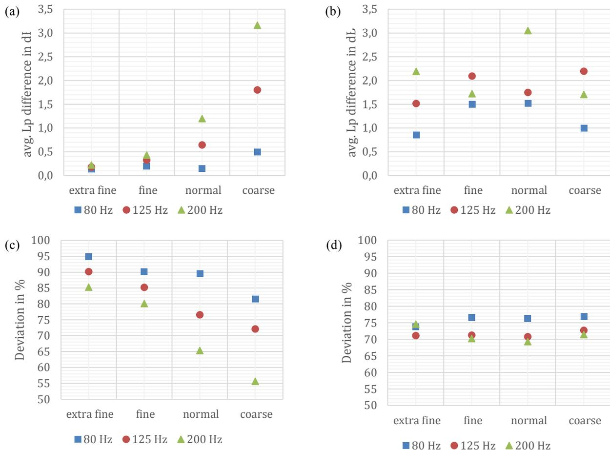
Figure 2. Illustration of the energy weighted average sound pressure level difference between the analytic solution and the FEM – simulations with different mesh densities in the sending room (a) and in the receiving room (b) Illustration of the average percentage of points in the FEM solution with less than 1 dB difference from the exact analytic solution in the sending room of all variations (c) and receiving room (d)
