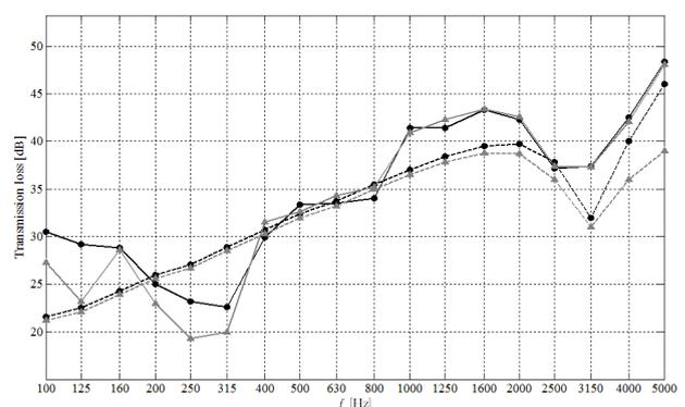
Figure 5. Measured (solid) vs predicted (dashed) sound transmission loss for the two kinds of panels tested.
