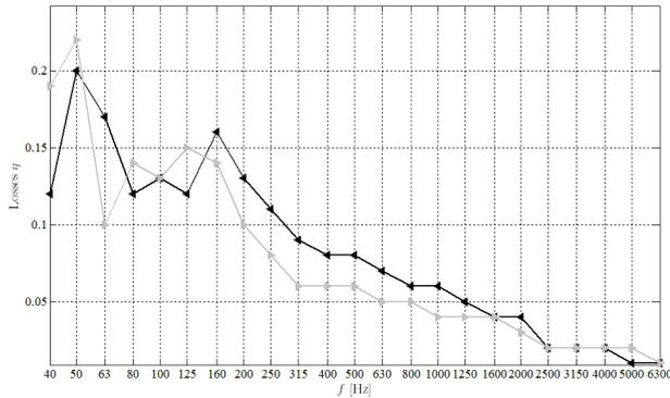
Figure 4. computed losses for the two panels tested (black – two laminates and wool inside, grey – two laminates and no wool inside).
