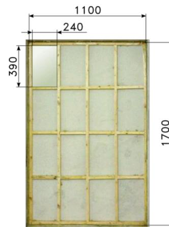
Figure 1. Layout of the ribs and main dimensions of the panel.
