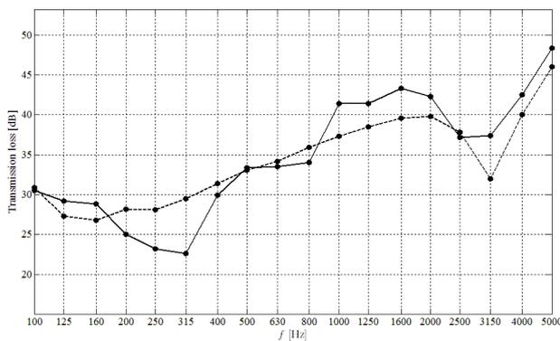
Figure 6. Predicted (solid) and measured (dashed) sound transmission losses for double panel with mineral wool in cavity.
