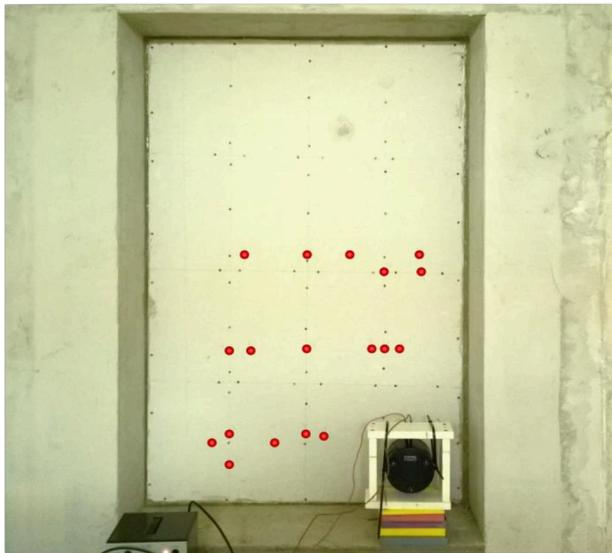
Figure 3. Measurement positions for the point mobility.
