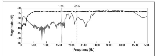
Figure 2. Frequency spectra of impulse responses obtained from a 3-D FDTD simulation of a 4-by-4 sonic crystal array. The black line is the spectra obtained from the simulation with no sonic crystal included for comparison. The vertical lines indicate the centre frequencies of the first theoretical band gaps associated with the first and second set of Bragg planes.
