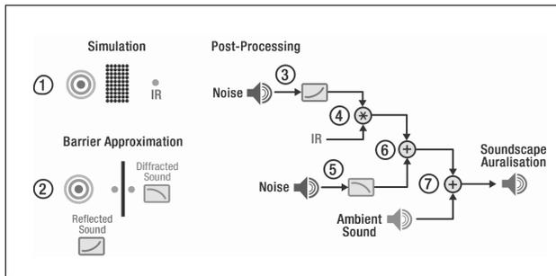
Figure 5. The step-by-step process used to auralise a sonic crystal barrier.
