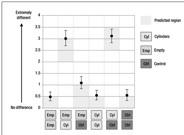
Figure 6. Results of paired perceivable difference test. *Ctrl* indicates the unprocessed soundscape material, *Emp* indicates the material was filtered with an impulse response obtained from an empty FDTD grid simulation, and *Cyl* indicates the material filtered with the sonic crystal cylindrical array.
