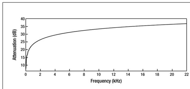
Figure 4. Frequency response of the amplitude envelope corresponding to a source and receiver on opposite sides of the thin rigid barrier pictured in Figure 3.
