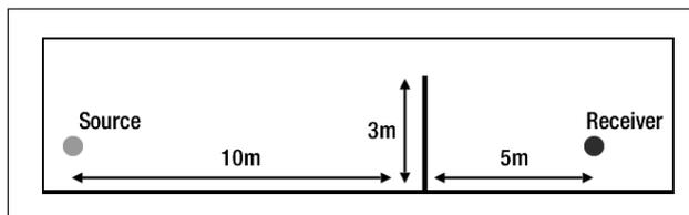
Figure 3. The source/receiver scheme of the virtual barrier. Note that the distances and barrier dimensions depicted in this example are arbitrary and can be adapted to a specific situation.
