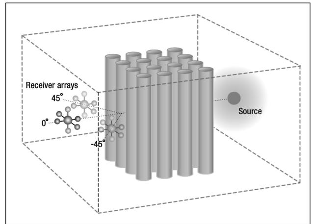
Figure 1. The FDTD simulation set-up used: a 4-by-4 sonic crystal array with a single sound source incident upon it and three receiver arrays, each consisting of seven adjacent grid points.
