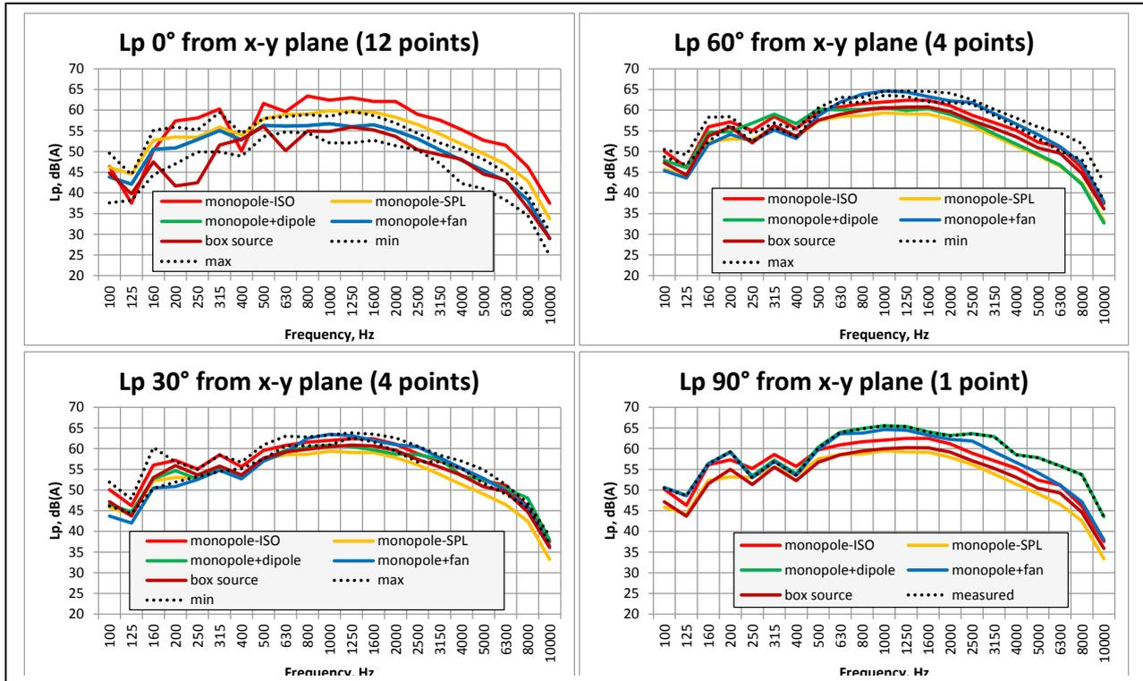
Figure 1 (above). Comparison of measured and calculated sound pressure levels for the directivity source tests. “Min” and “max” refer to measured levels.
