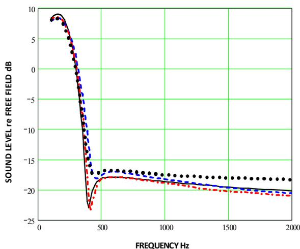
**Figure 7** Predicted Excess Attenuation spectra for source height 0.01 m, receiver height 1.5 m and range 100 m. Key to curves as for Fig.6.
