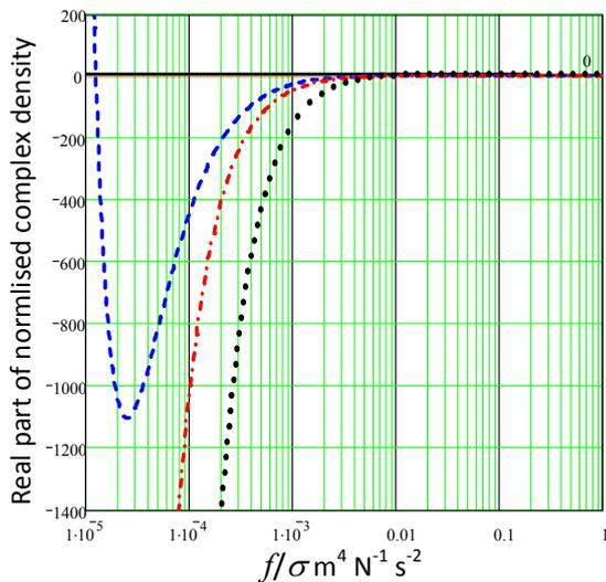
**Figure 2** Predictions of real part of normalised complex density as a function of frequency divided by flow resistivity for a 'grass-covered' ground (flow resistivity  $200 \text{ kPa s m}^{-2}$ , porosity 0.4, (hard-backed) layer thickness 0.03 m) according to slit pore (solid lines) Delany and Bazley (broken lines), three-parameter Miki (dotted lines) and modified Miki (dash-dot lines) models.
