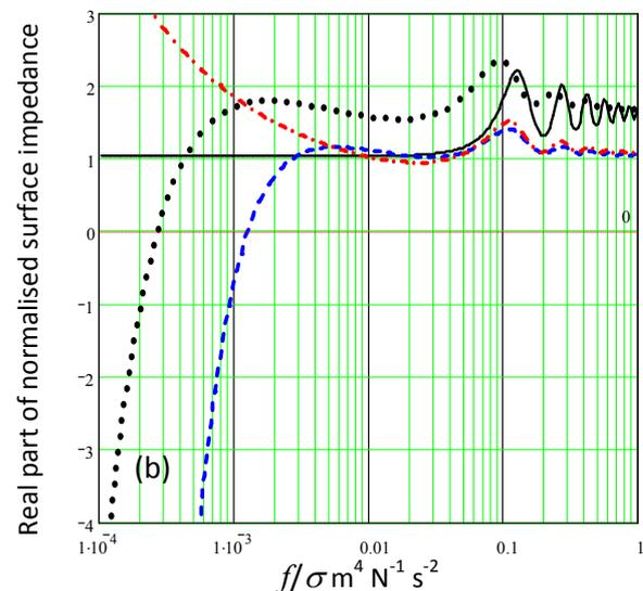
**Figure 1** Predictions as a function of frequency divided by flow resistivity of real parts of (a) normalised complex density for a 'snow-like layer' ground (flow resistivity  $10 \text{ kPa s m}^{-2}$ , porosity 0.7, (hard-backed) layer thickness 0.1 m) according to the slit pore model (solid line), Delany and Bazley model (broken line), three-parameter Miki model (dotted line) and modified Miki model [6] (dash-dot line).
