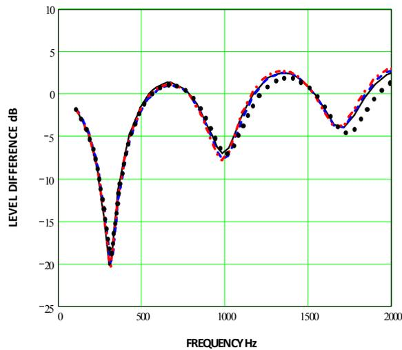
**Figure 6** Predictions of Level Difference spectra (allowing for moderate turbulence) for source height 1 m and receivers at heights of 1 m and 0 m at a horizontal distance of 4 m from the source. Predictions use the slit pore layer model (black continuous line), Delany and Bazley layer model (broken blue line) modified Miki model (red dash-dot line) and three parameter Miki layer model (black dotted line).
