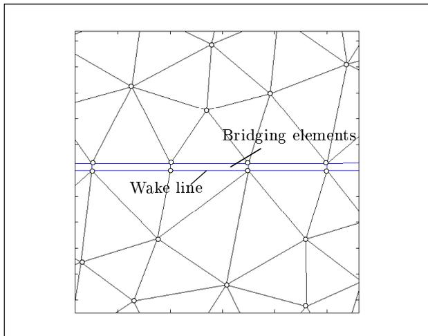
Figure 1. Bridging elements on the shear layer.
