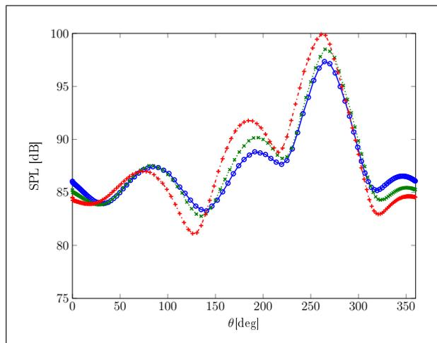
Figure 5. Sound pressure level.  $f = 100$  Hz,  $R_{fp} = 2.5L$ .  $M_\infty = 0.3$  (solid - marker: +),  $M_\infty = 0.2$  (dotted - marker: x) and  $M_\infty = 0.1$  (dashed - marker: o). Scattering by a NACA 0012 from a monopole source with a non-uniform mean flow, dependency on the Mach number.
