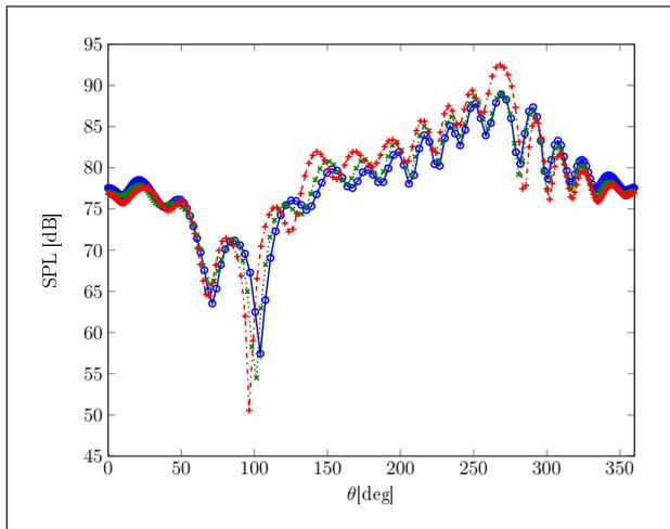
Figure 6. Sound pressure level.  $f = 500 \text{ Hz}$ ,  $R_{fp} = 2.5L$ .  $M_\infty = 0.3$  (solid - marker: +),  $M_\infty = 0.2$  (dotted - marker: x) and  $M_\infty = 0.1$  (dashed - marker: o). Scattering by a NACA 0012 from a monopole source with a non-uniform mean flow, dependency on the Mach number.
