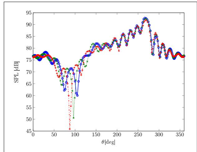
Figure 8. Sound pressure level.  $f = 500 \text{ Hz}$ ,  $R_{fp} = 2.5L$ .  $\alpha = 10^\circ$  (solid - marker: +),  $\alpha = 4^\circ$  (dotted - marker: x) and  $\alpha = 0^\circ$  (dashed - marker: o). Scattering by a NACA 0012 from a monopole source with a non-uniform mean flow, dependency on the angle of attack.
