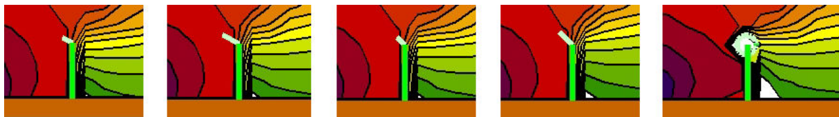
Figure 2. Noise barriers of various configurations of examination II.
